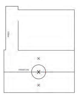
10. Snap a line across the length of the room, perpendicular to the primary line, connecting the marks. This line is your secondary line, and should be perpendicular to the primary line.
