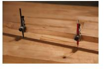
or attached to a beam. They are used in situations where a traditional compass is too small for the area, which makes them ideal for wood flooring. The beam should be a minimum of 4' in length. A longer beam will be beneficial for larger floor spaces.
