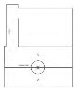
9. Move the trammel point end to the opposite location where the circle intersects the primary line. Use the marking point of the trammel to draw an arc above and an arc below the primary line, as near to perpendicular to the center mark point "C" as possible, crossing the marks made in the previous step.
