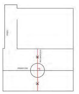
D. You can also square a room or check that your lines are perpendicular by using the 3-4-5 rule.
