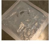
the presence of capillary moisture in concrete. This test can provide useful information, but should NOT be used to determine whether a floor should or should not be installed.
