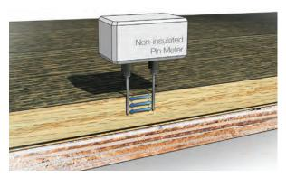
i. Non-insulated pins will read as deep as they are inserted and will report the highest value of resistance through the entire depth of the pins.
