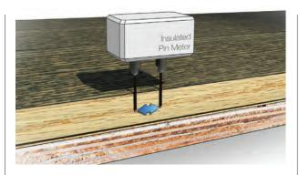
ii. Insulated pins are typically available in many different lengths, from 1"-3", and are normally used with a slide hammer extension. Insulated pins only measure the resistance at the uninsulated tips of the pins, allowing one to evaluate the moisture gradients through the sample of flooring, subflooring, or the entire flooring system.
