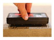
gypsum cement, and other floor slabs and screeds. It is a nondestructive testing method. These tests should be used to evaluate the surface of the concrete and to determine where to place other quantifiable tests. These tests provide useful information, but should not be used on their own to determine whether a floor should or should not be installed unless otherwise directed by the flooring manufacturer.
