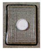
calcium chloride. The results of this test give quantifiable values.
