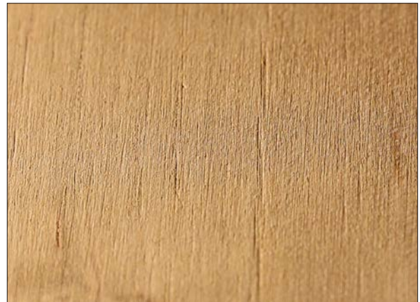
This shows the deep scratches left behind from the 40 grit when more than one grit has been skipped in the sanding sequence, moving straight from 40 grit to 100 grit.
