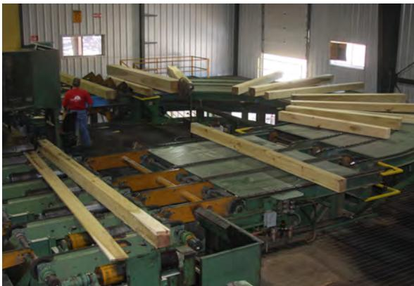
The square logs are next cut into wood slabs at a predetermined thickness, maximizing the usable lumber. The slab edges are then trued and trimmed square, creating what we typically call a lumber board.
