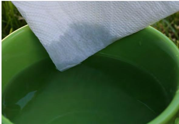
Capillary action refers to the ability of water to travel up against the pull of gravity through a porous material. One common example of this action is water “wicking” up through a paper towel, following the direction of the paper fibers (as seen in the photo). Although not as serious as bulk water movement, capillary forces are both powerful and rather secretive, since they often work in the dark of a crawlspace, causing significant damage to a building without the occupant’s knowledge.
