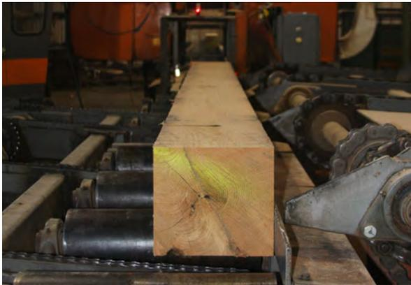
For sawn or sliced material, the rounded edges are then removed to produce a square log called a cant.
