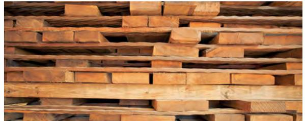
After sorting, boards are stacked to facilitate air movement and begin the air-drying process. This is accomplished by placing small, thin boards called "stickers" between each stacked layer of wood. This maximizes air movement, which helps to bring the moisture content of the lumber into equilibrium with its surrounding environment. The temperature, humidity and airflow will influence the time needed to reduce moisture content of the wood. The goal is generally to reach 18-30% moisture content.
